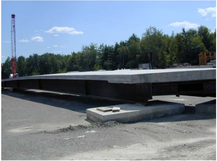
Figure 10. Inverset TM deck unit stored at the precast plant. Note camber induced during the casting operation.
