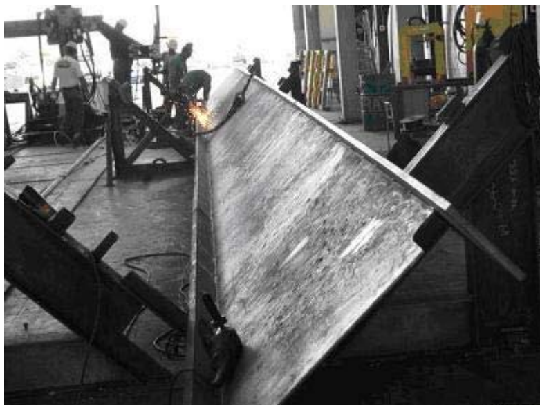
Figure 2.2.7. Girder Fabrication at Stinger Welding
