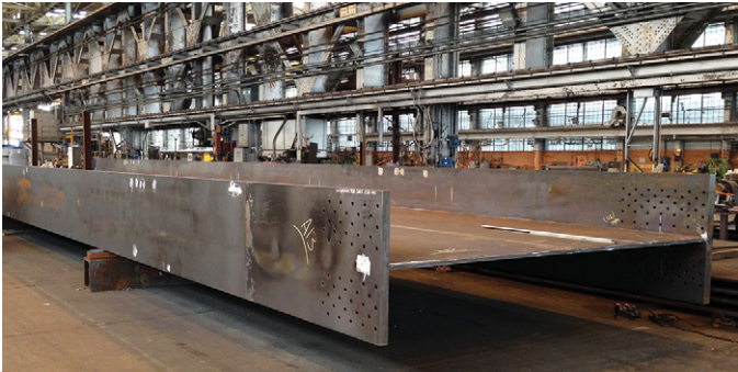
Crews demolished the Pfeiffer Canyon Bridge in March following torrential rains in February that damaged the span. Its replacement is expected to open in mid to late September, using 15 steel girders being constructed in Vallejo, bottom right. Each girder is 63 feet long and weighs 56 tons. They will be connected on site, then rolled into place across the canyon using strategically placed winches and cables.
