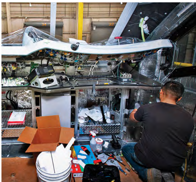
A Siemens employee works on a Charger display panel equipped with a diagnostics system designed to show the severity of faults detected within the locomotive.
