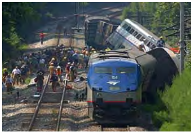
Derailment from warped tracks due to extreme heat. Upward slab movement and shattering at a joint or crack.
