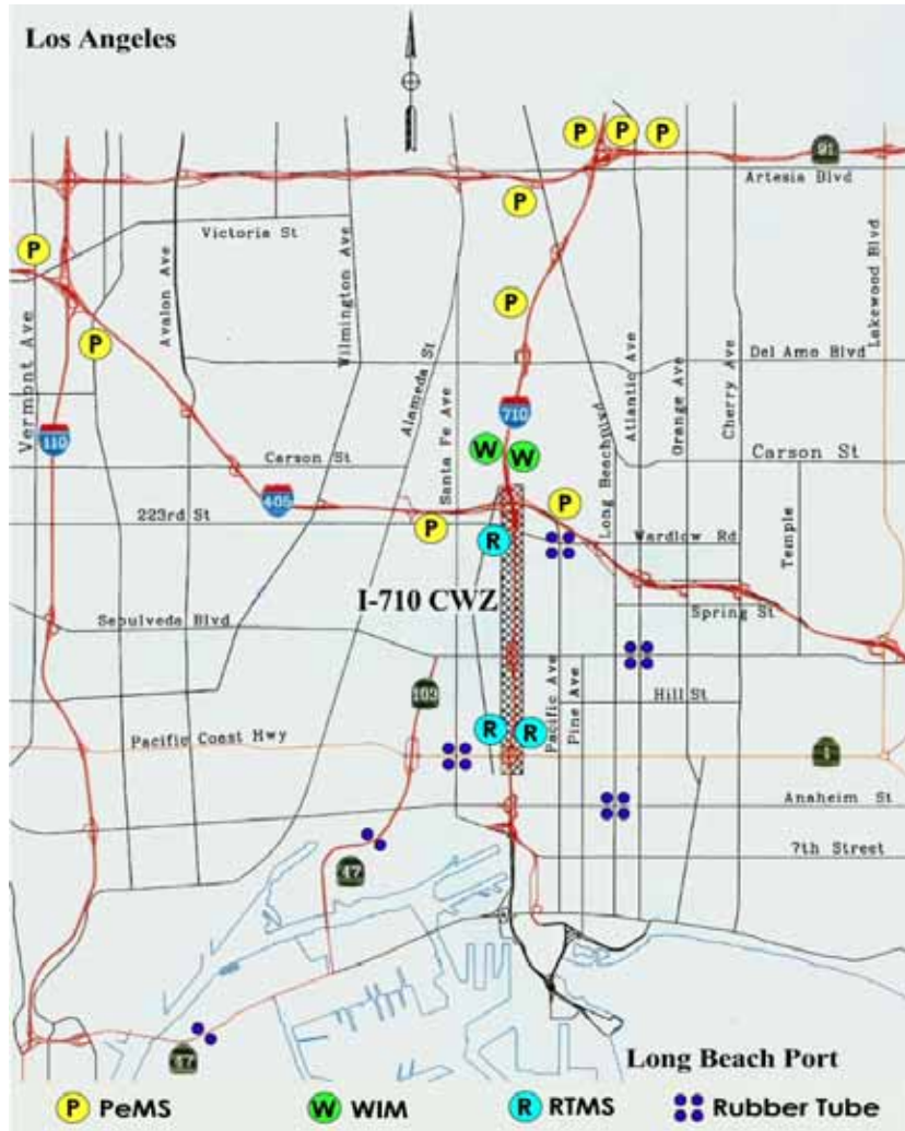
Figure 4. Traffic study area showing locations of traffic monitoring devices
