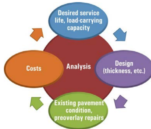
Figure 110-3: Interrelationship of pavement design elements 2
