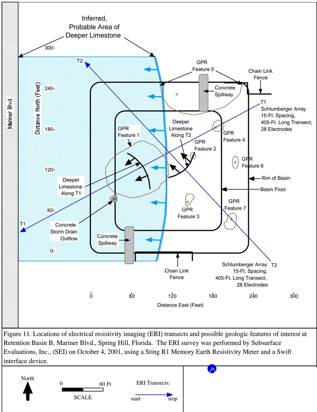
Figure 11. Locations of electrical resistivity imaging (ERI) transects and possible geologic features of interest at Retention Basin B, Mariner Blvd., Spring Hill, Florida. The ERI survey was performed by Subsurface Evaluations, Inc., (SEI) on October 4, 2001, using a Sting R1 Memory Earth Resistivity Meter and a Swift interface device.
