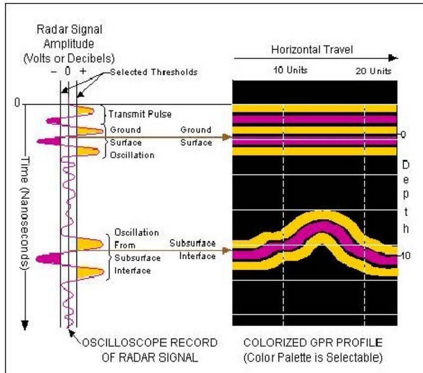
Figure 2: Example of Ground Penetrating Radar Profile
