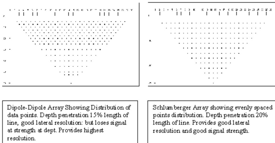
Figure 3: Comparison of Dipole-Dipole and Schlumberger Arrays
