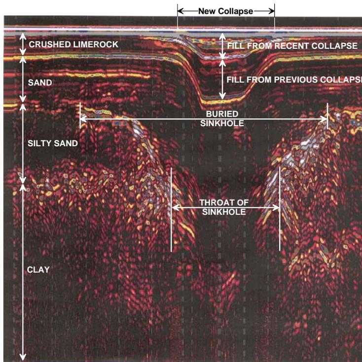
Ground penetrating radar (GPR) survey of a newly formed sinkhole in the northbound lane of Thonotosassa Road about 4 miles north of I-4, east of Tampa, Florida. The new sinkhole developed January 00, 2001, and was 00 feet wide. The GPR survey was performed using a SIR-2000 digital control unit and a 500 MHz antenna. Original range was 102 nanoseconds. Surveyed January 00, 2001, by Michael Garman, P.E., P.G., and Scott Waddell, SEI.
