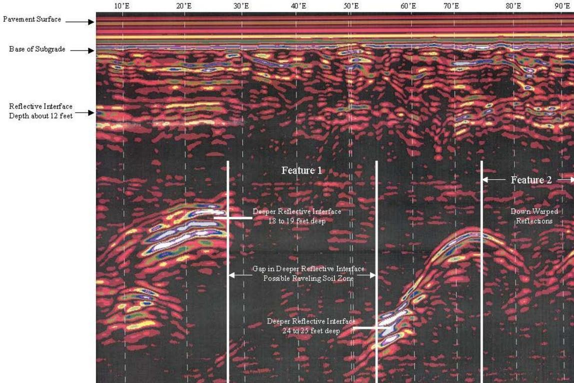
Figure 7: GPR Profile Showing Karst Features beneath State Route 54
