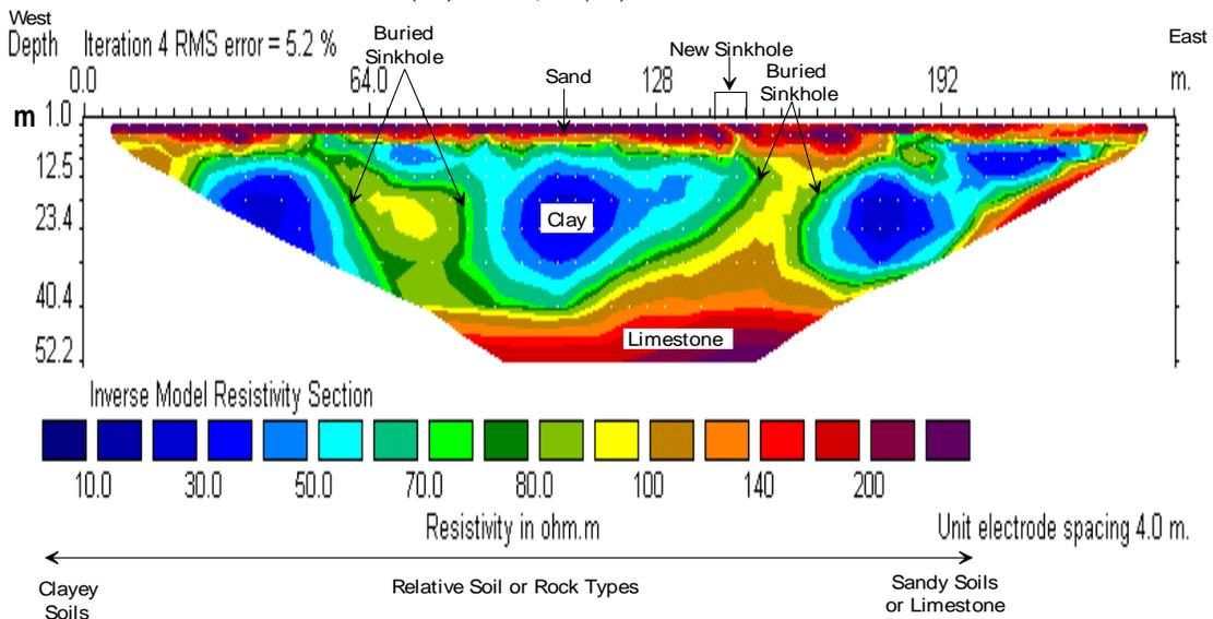
Figure 8: ERI Profile Showing Karst Features beneath State Route 54
