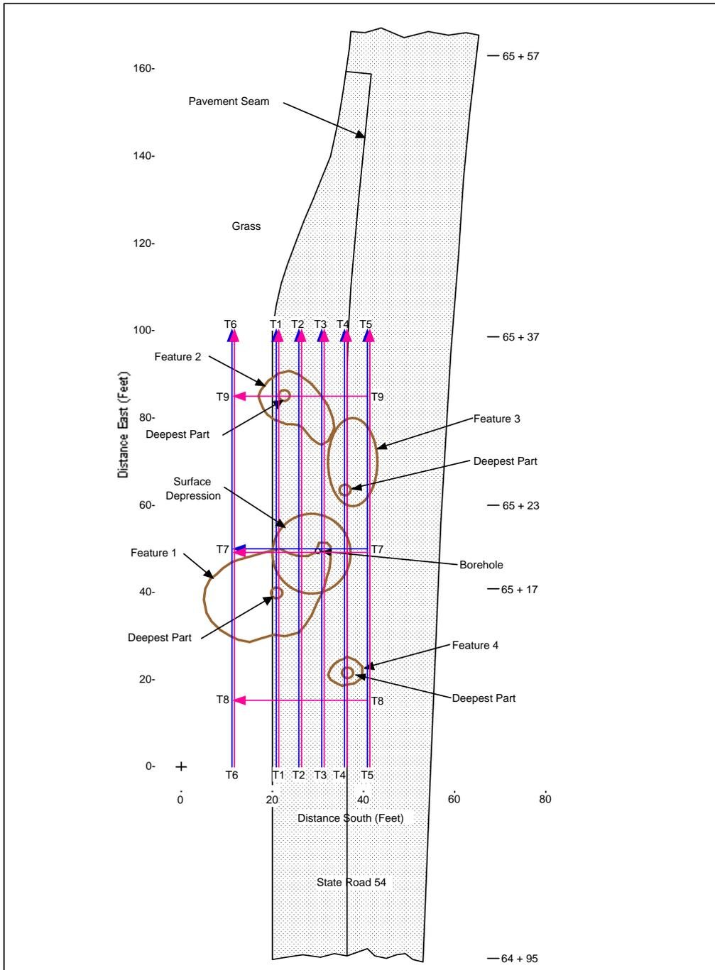
Figure 6. Locations of ground penetrating radar (GPR) transects and features of interest at a new depression along S.R. 54, Land O' Lakes, Florida. The GPR survey was performed by Subsurface Evaluations, Inc. (SEI), on March 13, 2001, using a SIR- 2000 control unit, a 100-MHz antenna, and a 500-MHz antenna.
