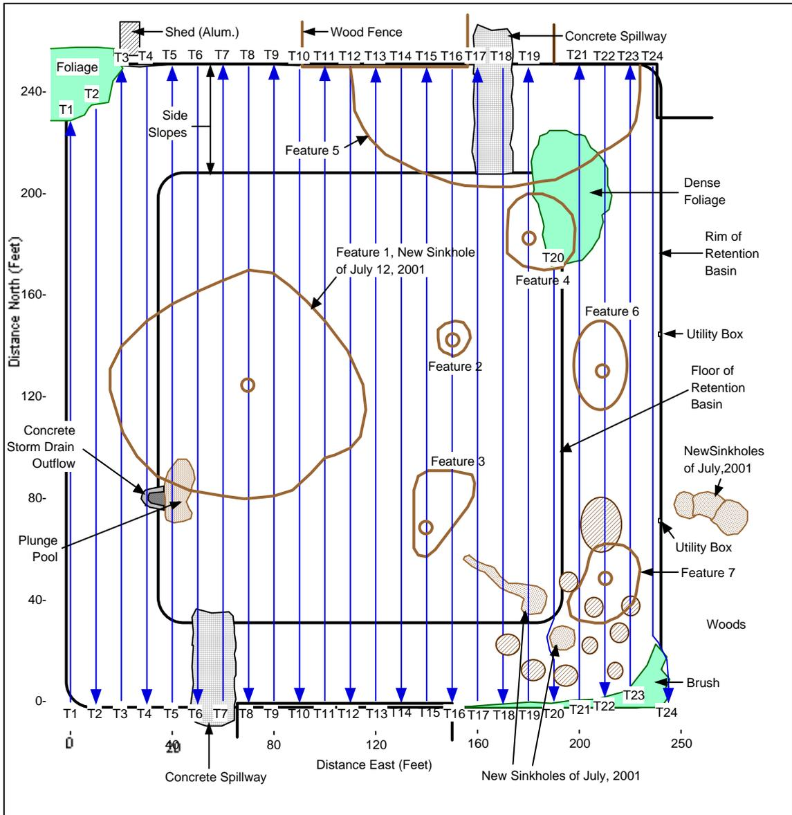
Figure 10. Locations of ground penetrating radar (GPR) transects, buried sand-filled depressions, and new sinkholes as of September 25, 2001, at Retention Basin B, Mariner Blvd., Spring Hill, Florida. The GPR survey was performed by Subsurface Evaluations, Inc. on September 25, 2001 using a SIR-2000 Digital Control Unit and a 400-MHz antenna.
