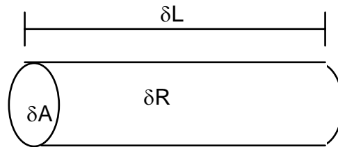
Figure 1. Resistivity is defined based on the change in resistance \delta R for a given change in length \delta L and cross-sectional area \delta A of material.
