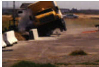
8000-kg Truck Impacting Type 732 Bridge Rail
