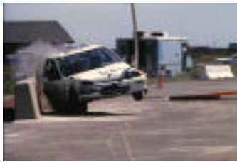
820-kg Sedan Impacting Type 732 Bridge Rail
