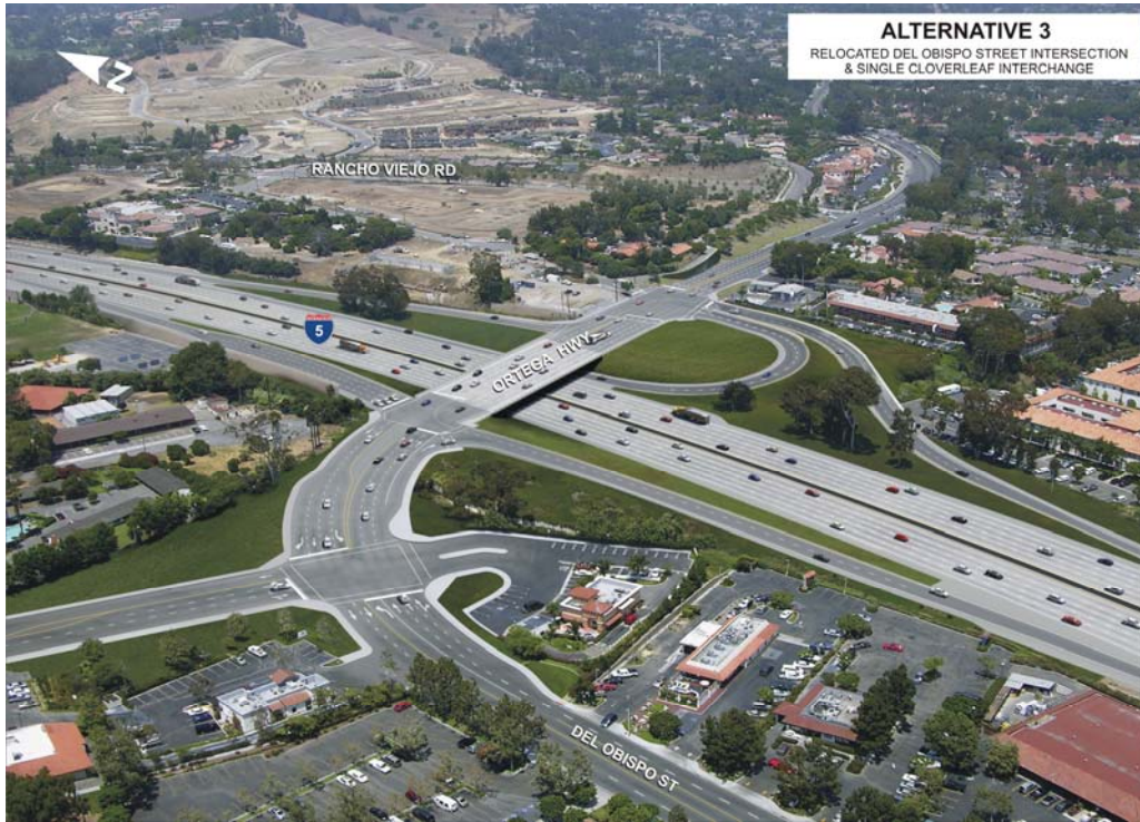
Figure 2.1.5-2 Alternative 3 Aerial View of Proposed Improvements
