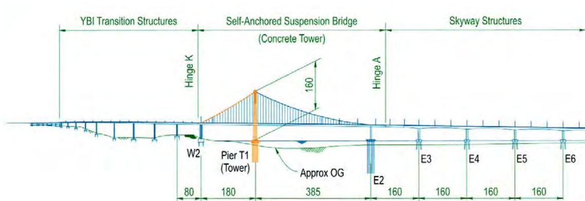
Figure 3-2. SAS with Concrete Tower
