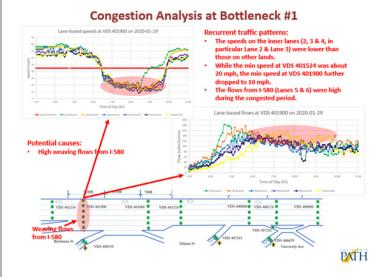
Image 1: Bottleneck congestion analysis on I-580, the researcher took data from detectors on the freeway to reconstruct the flow of vehicle to identify congestion
