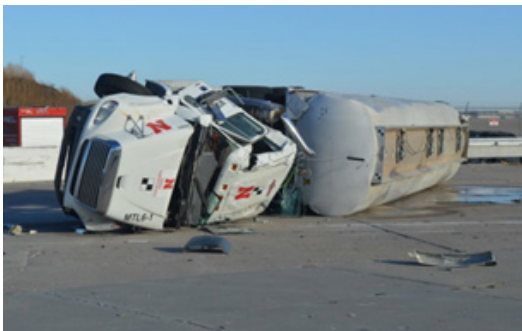
Image 2: Test No. MTL6-1 MASH TL-6 Crash Test
