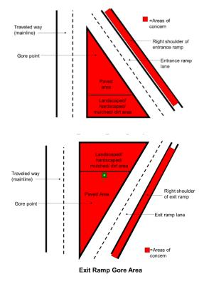
For stationary operations in gore areas, ramp closures and barrier vehicles should be placed to ensure Maintenance force safety in addition to required lane or shoulder closures on the through lane. On and off ramps should be closed per Standard Plan T14. Barrier vehicles shall be parked across closed ramp(s) to prevent traffic from going around the cones and signs. Special instances may require a deviation. If a deviation is required, please see Section 8.07 Changing Chapter Standards.
