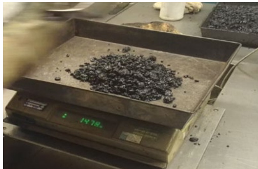
FIGURE 3 Monitor and Adjust Each Box Increment Size to Achieve the Desired Final Test Sample Weight
