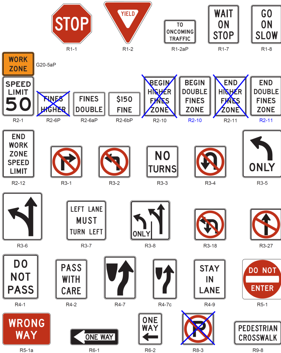
Figure 6F-3. Regulatory Signs and Plaques in Temporary Traffic Control Zones (Sheet 1 of 2)
