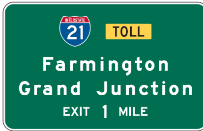
Figure 2F-5. Examples of Guide Signs for Entrances to Toll Highways or Ramps
