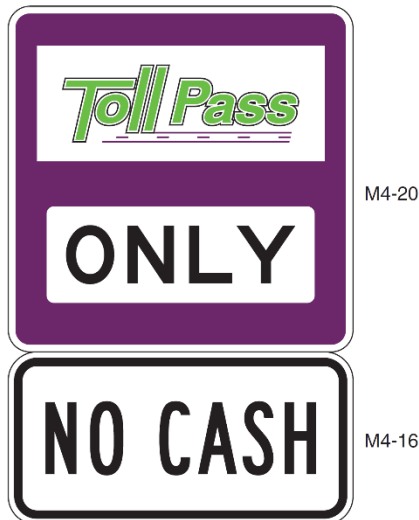
Figure 2F-4. ETC Account-Only Auxiliary Signs for Use in Route Sign Assemblies
