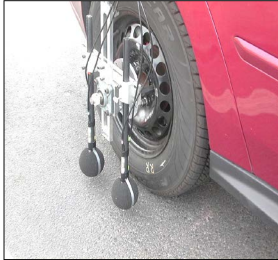
Figure 6.1-5. Typical Research Setup Quantifying Tire-Pavement Interface Noise Level.
