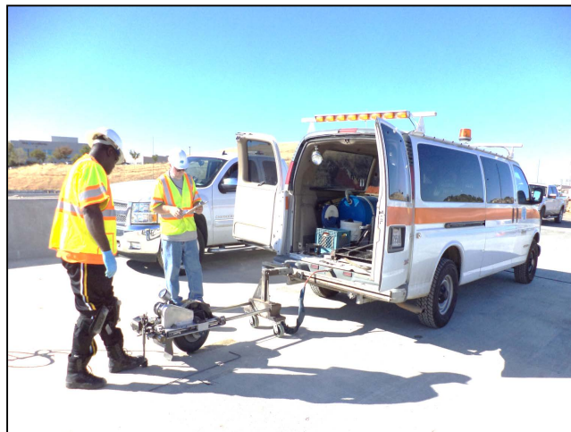
Figure 6.1-2. Coefficient of Friction Testing per California Test 342 .
