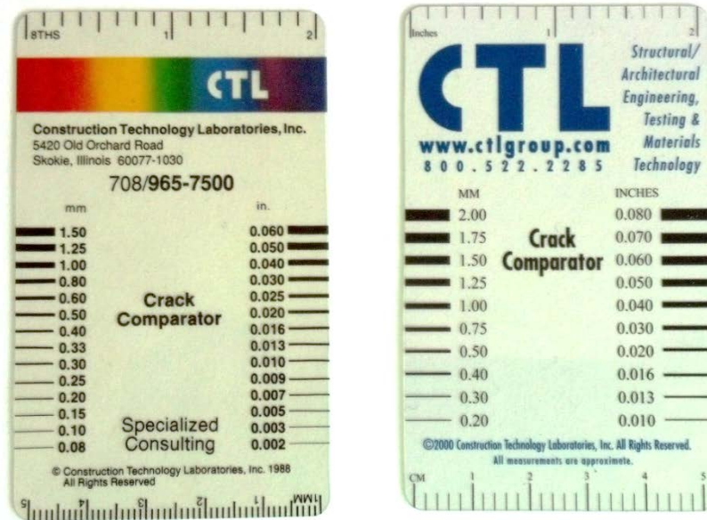
Figure 6.1-3. Crack Comparator Makes Checking Crack Width Easier.
