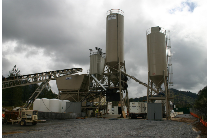
Figure 4-1. Basic Batch Plant Shows Aggregate, Cement and Supplemental Cementitious Material Storage, Conveyor Feed System, Chemical Admixture Tanks and Dust Collector.
