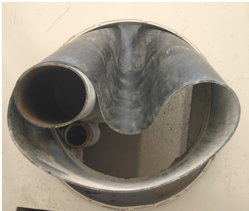
Figure 4-14. Sock Used at a Truck Mixer Charging Chute.
