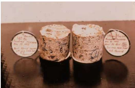
Figure 8. Pull-Out Test Cores
