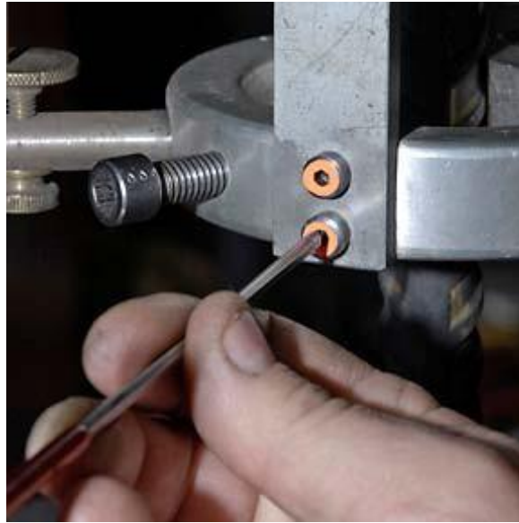
FIGURE 2a. Close up of the removal of the hex socket bolts before testing.
