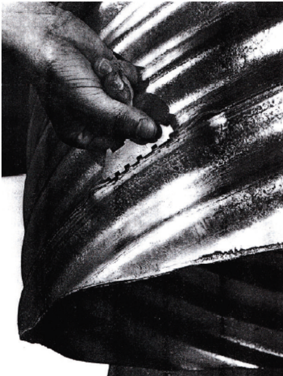
FIGURE 8. Minimum Acceptable Distance Between Cup Tests
