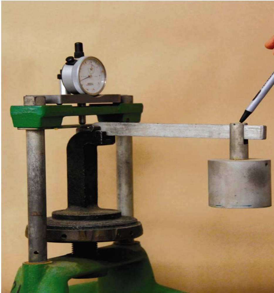
FIGURE A3. Expansion Pressure Device Calibration Verification Procedure
