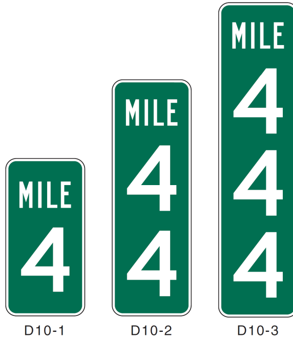
Figure 2H-2. Reference Location Signs
