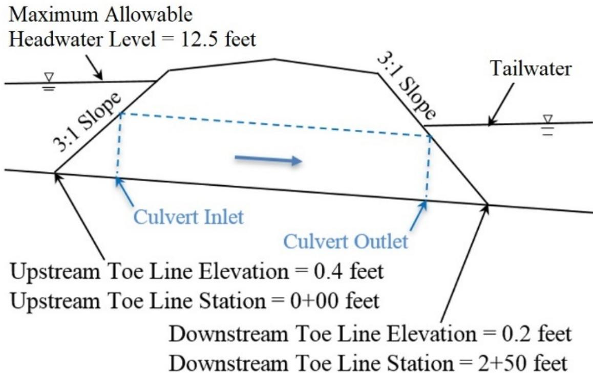
Step 1: Obtain the Tailwater Depth for the corresponding discharge to represent a 1% probability of exceedance event
